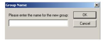
Enter the name for the new group in the **Group Name** window. The new name can be over 40 characters long, but the display in the **Group Setup** window will not display more than 40 characters, and the window in the **Presets** tab will only display 17 characters.
