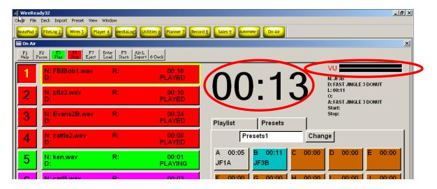
The VU meter in the upper-right corner of the window displays the audio levels being played from the 10 decks or the Presets.
